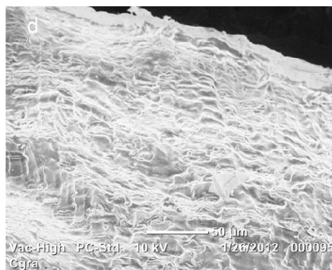
Figure 6-8. SEM images of (a) and (b) raw biomass, 3-in. minus corn stover; (c) and (d) pelleted corn stover.
