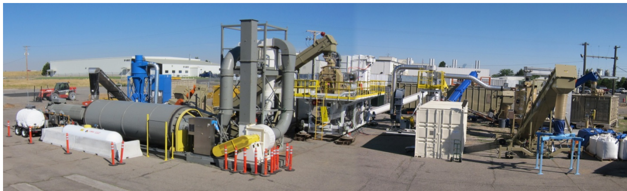
Figure WO–4. The Feedstock PDU is a flexible research system developed to test feedstock preprocessing, formulation, and densification processes, collect process data, and produce large quantities of advanced feedstocks for conversion testing.
