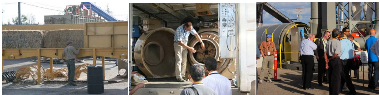
Figure WO–5. Feedstock formulation was demonstrated using four types of biomass (corn stover, switchgrass, pine, and eucalyptus) processed in a 1-1-1-1 ratio and densified into a pelletized product.
