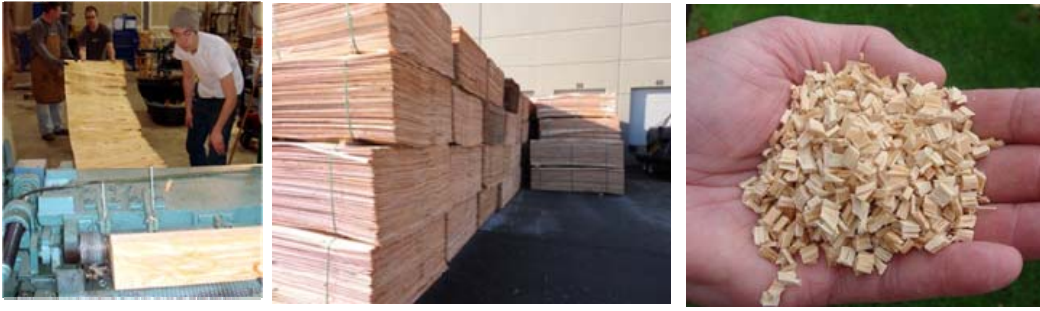
Figure 2–8. Veneering raw wood (a), stacked veneer sheets (b), and final Crumbles® product (c).
