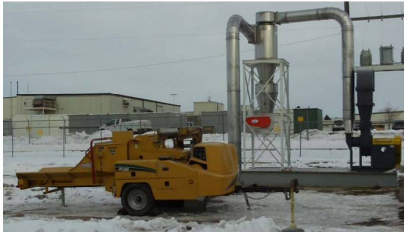
Figure 2–3. Grinder setup to test pneumatic conveyance of the test feedstocks.
