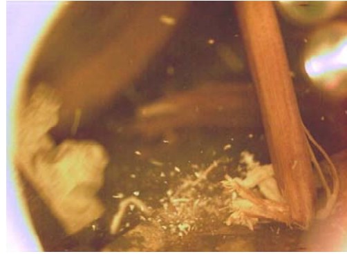
Figure 2–6. High-speed video analysis revealed that fines generation in hammer-mill grinding largely results from non-fibrous tissues that disintegrate into small particles when they are impacted with the rotating hammers and/or fixed shear plates.
