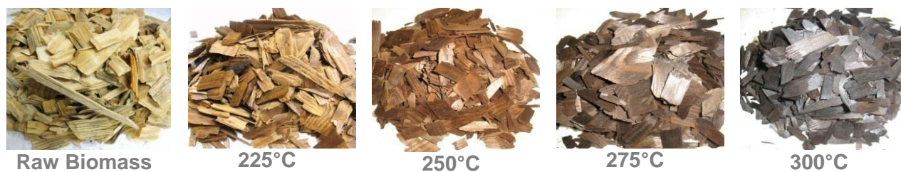
Figure 3–2. Resultant product torrefied in the range of torrefaction (200 to 300°C) (Phanphanich & Mani 2010).
