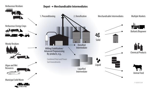
Figure 16. Schematic of an Advanced Feedstock Supply System, including distributed depots.
